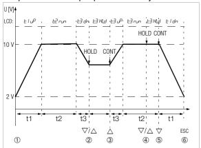
Ramp parameters: output quantity: U (range of 0 ... 15 V),  $5 \pm Rr = 2 \text{ V}$ , Erd = 10 V, Erd
