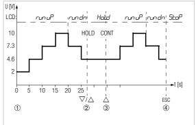
**Interval parameters:** output quantity: U (range of 0 ... 15 V), S & H = 2 V, E = 10 V, number of interval steps = 3, E = 5 S, E = 10 V, E
